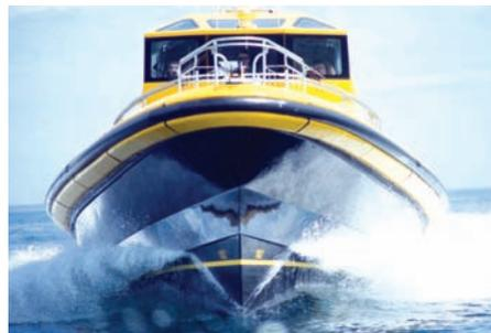
*The 'Kestrel's' beak bow lowers into the water in rough weather via the vessel's trim tab system. This lowering adjusts the longitudinal trim to increase speed and decrease drag*
