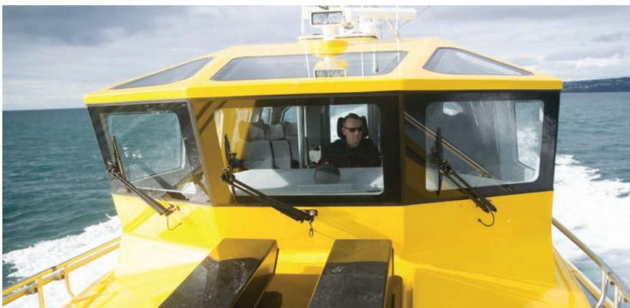
*To reduce pilot fatigue, the vessel's resiliently mounted wheelhouse features vibration dampening qualities as well as noise levels below 70 decibels*
